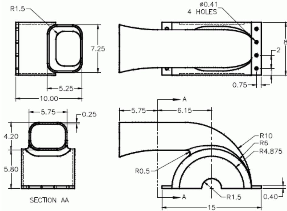
Figure 3 Dimensions of the Upper Housing
