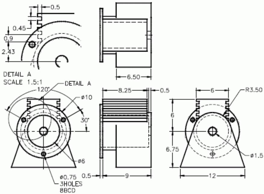
Figure 6 Dimensions of the Motor
