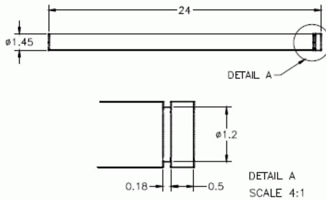
Figure 8 Dimensions of the Shaft
