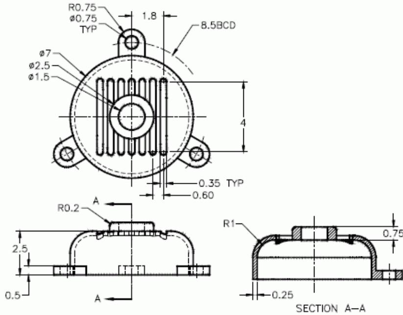
Figure 7 Dimensions of the Cover
