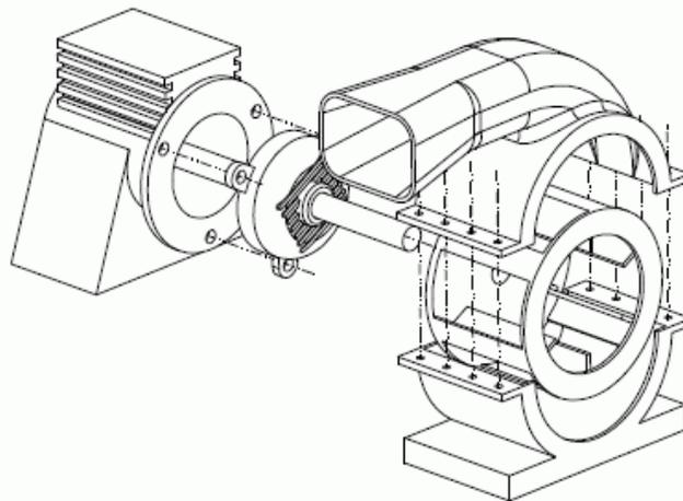
*Figure 2 Exploded view of the Motor Blower assembly*
